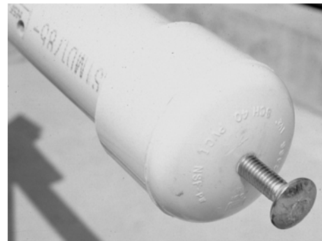
Adjustment carriage bolt in PVC end cap
