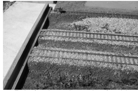
Ends of tracks running to edge of module with boards fastened to end of module to protect ends of tracks
