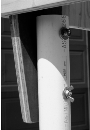
PVC leg attached with mounting hardware
