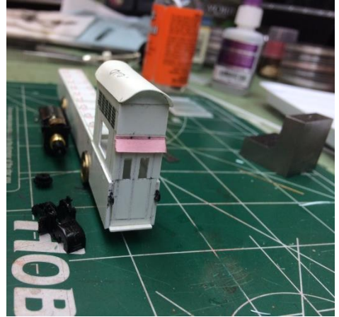
The canopy above the doors is made from a used Micro-Mark paper bad order tag. The black on the side of the cab above the windows are Micro-Mark louver decals.
