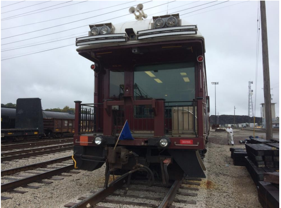
PIC B. The blue flag is protecting the platform end of NS track geometry car in Luther yard.
