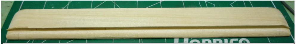
PIC B After the floor length was finalized the roof was cut to length to match and the running end sanded to shape.
