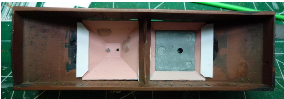
Picture H-2 Securing the silos and weighting the car
