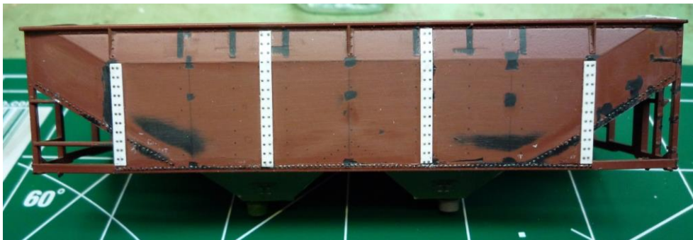
Picture I. Added bolt plates decal rivets
