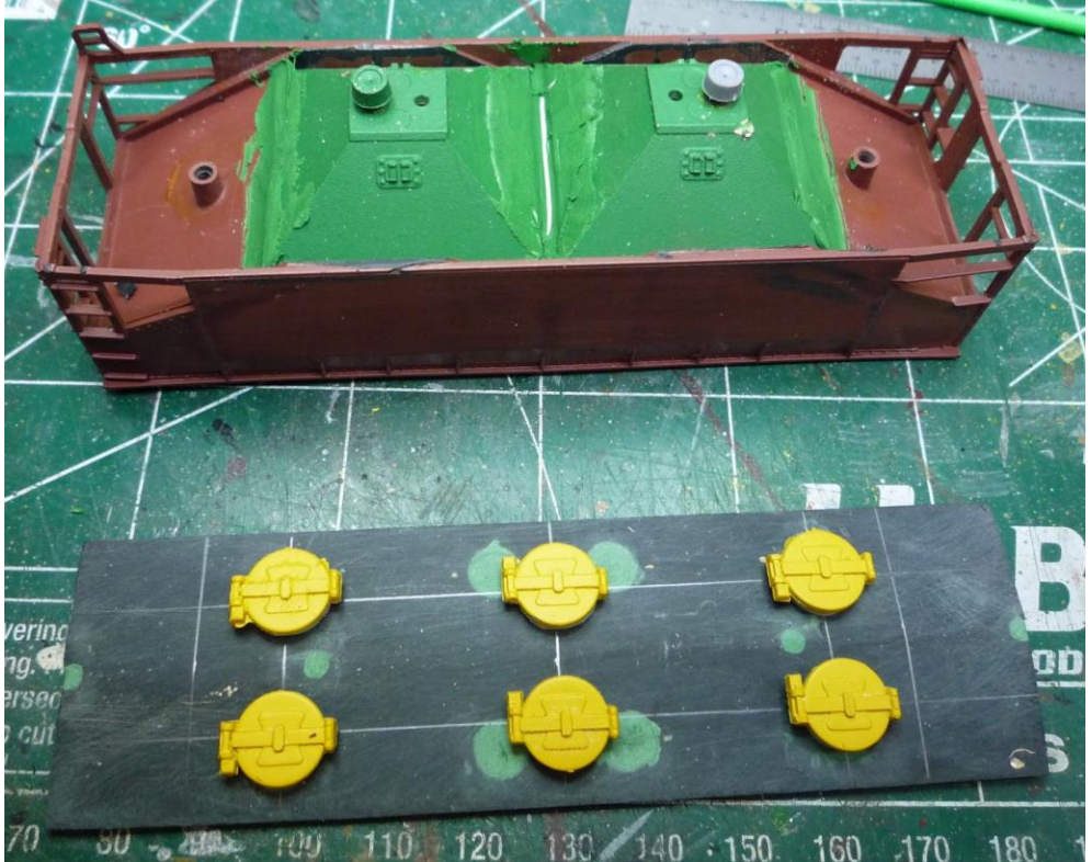
Picture F. The new hatches on the roof and the new silos under the car.
