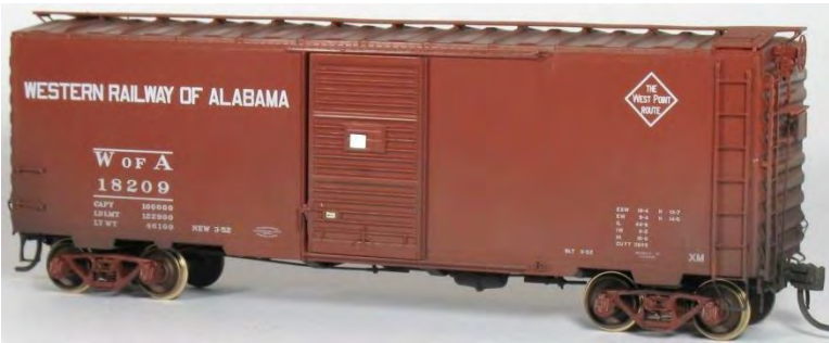
Photo 6. The Kadee factory-painted model, weathered but prior to application of HO scale car cement to the roof.
