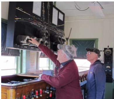
Photo 7 George Detwiler (at right), one of the principal men responsible for moving the tower to its present site and restoring the interlocking machine, assists a railfan in setting a timer to clear the interlocking during a simulation. George is a former railroad employee and understands the interlocking logic well, and is a very patient instructor.
