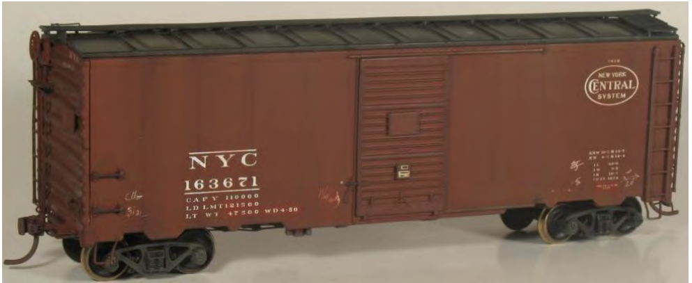
Photo 10. Central acquired a large number of 1944 ARA-design box car with 10-foot, six-inch interior height, 4-4 Improved Dreadnaught ends, and Barber S-2 trucks in several series. This model represents a car from Lot 743-B (see Photo 11 below). The model is equipped with Improved Youngstown doors but the prototype series was delivered with pre-war Youngstown doors. John Golden photo.
