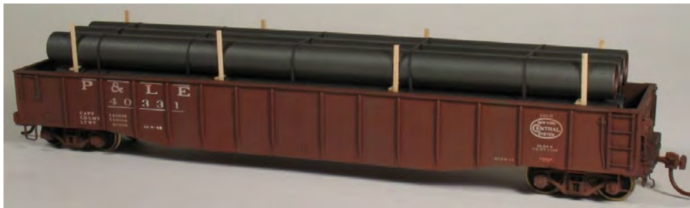
Photo 3. P&LE 40331 represents one of 6,000 Greenville-design gondolas built for NYC subsidiary Pittsburgh and Lake Erie in May, 1945. P&LE received 6,000 cars in five lots, the last of which were the 40000-40999 series, Lot 740-G, built by NYC's Despatch Shops of East Rochester, New York. These were rugged cars with wood floors and drop ends, and served the NYC lines through the Penn Central merger and beyond. Photo by John Golden.
