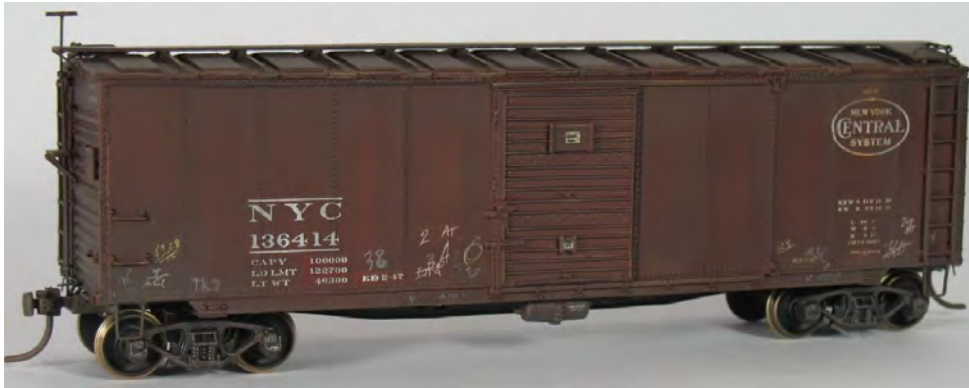
Photo 20. NYC 136414 is a model of a 1916-design all-steel box car. Central owned thousands of cars to this design in multiple lots and the cars appeared in a wide number of number series. Many were modified or rebuilt during the pre- and post-WWII era. This car is similar to the thousands of USRA all-steel box cars Central built during the same period. Photo by Kirsten Golden.
