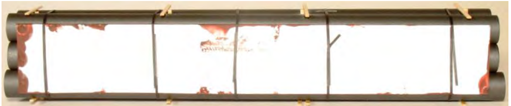
Photo 5. This photo shows the bottom of the load so you can see how the simulated wire bands are attached. They are simply wrapped snugly around the pipe load and then taped to the bottom of the false floor. Photo by John Golden.
