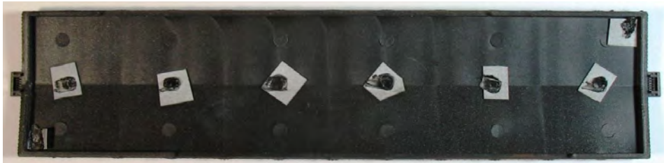
Photo 12. The underside of the Branchline roof, showing the tabs fixed to small pieces of styrene and then melted in place. This technique is time-consuming but allows the roof to flex, and eliminates the problem of adhesives filling the holes in the running board. Photo by Kirsten Golden.
