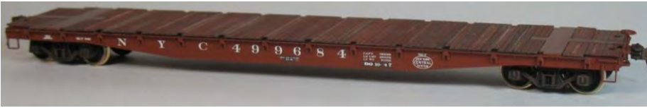
Photo 16. NYC 499684 is a model of a 70-ton 53' 6" AAR flatcar that was derived from a Greenville Car Company design. Central built 1,000 cars at Despatch Shops beginning in November, 1942, to help handle wartime traffic. This particular lot, 721-F, included cars in the 499300-499599 series. An additional 300 cars were delivered 1943 with 200 going to NYC and 100 going to NYC subsidiary Indiana Harbor Belt and the remainder were delivered in 1950. Photo by Kirsten Golden.
