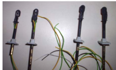
Signals with light emitting diodes installed before (left) and after (right) painting of the wires and backs of diodes.
