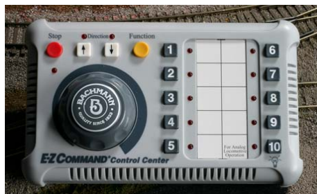
Motive power and control system are by Bachman. The E-Z Command basic throttle is supplemented by a second walk-around throttle. Land forms are Sculptamold over rigid foam insulation board.
