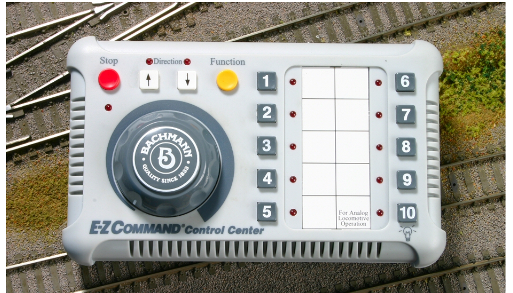
A Bachmann E-Z Command DCC Throttle is used to control the engines on this layout.
